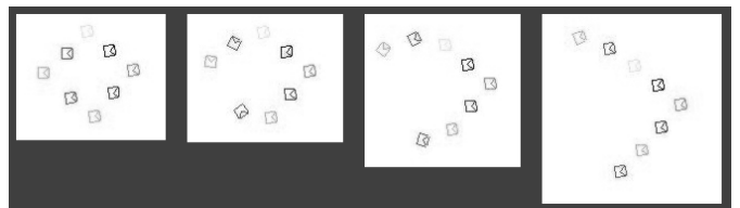
Fig. 8. Example: 8 robots switching from a diamond to a wedge.
