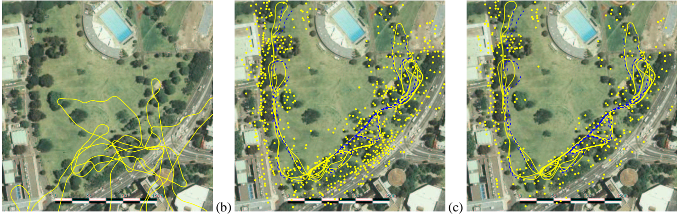
Figure 1: FastSLAM 2.0 applied to the Victoria Park benchmark data set. (a) Raw vehicle odometry (b) FastSLAM 2.0, M=1 particle (c) FastSLAM 2.0 with dynamic feature management.
