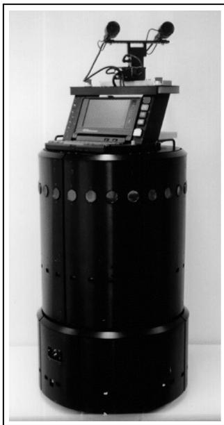
Figure 1. The robot RHINO, an RWI B21.
