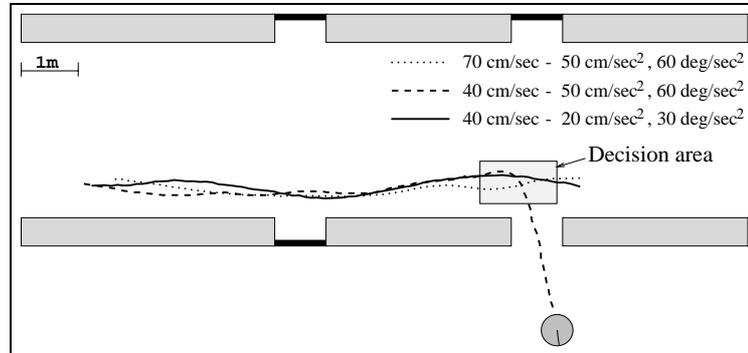
Figure 20. Trajectories chosen for different dynamic parameters
